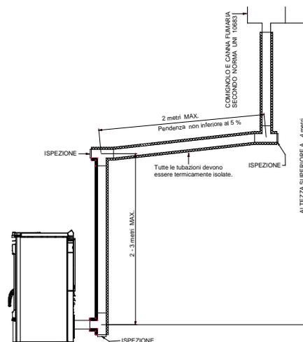
These openings are essential to allow for the removal of ash and unburned products which tend to accumulate along the discharge path. The appliance functions with the combustion chamber in a vacuum, while the discharge of smoke to the flue outlet has a slight pressure, consequently it is imperative to ensure that the discharge system is hermetically sealed.
